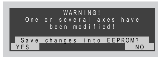
Fig. 1.15 — Save screen for axis modifications.
